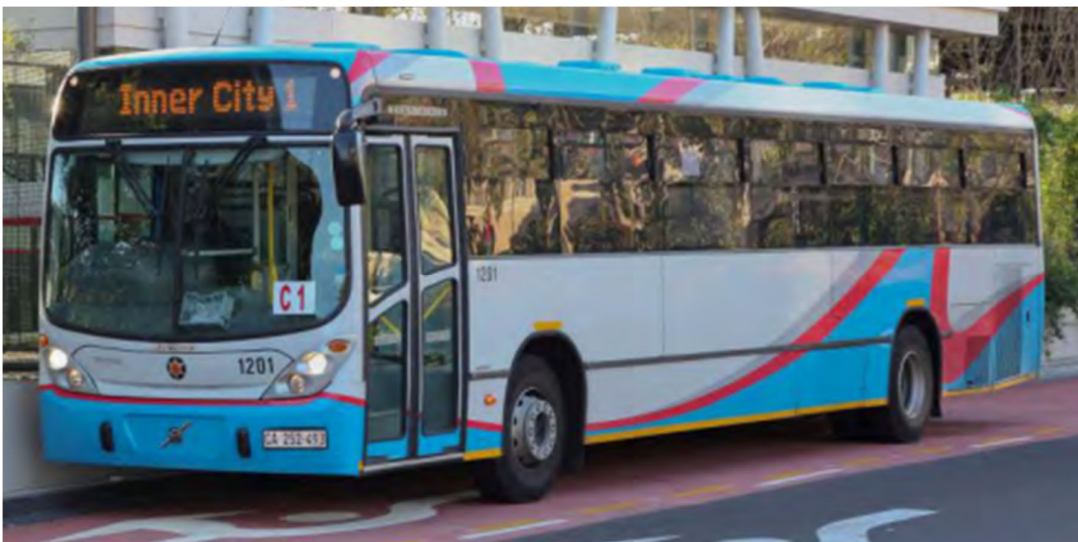
Figure 2-2: Example of a high floor 12m bus
