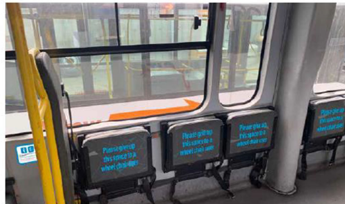
18. Wheel Chair User Stencil: ±w 200mm x h 200mm 16. Red Seat: w 145mm x h 118mm
