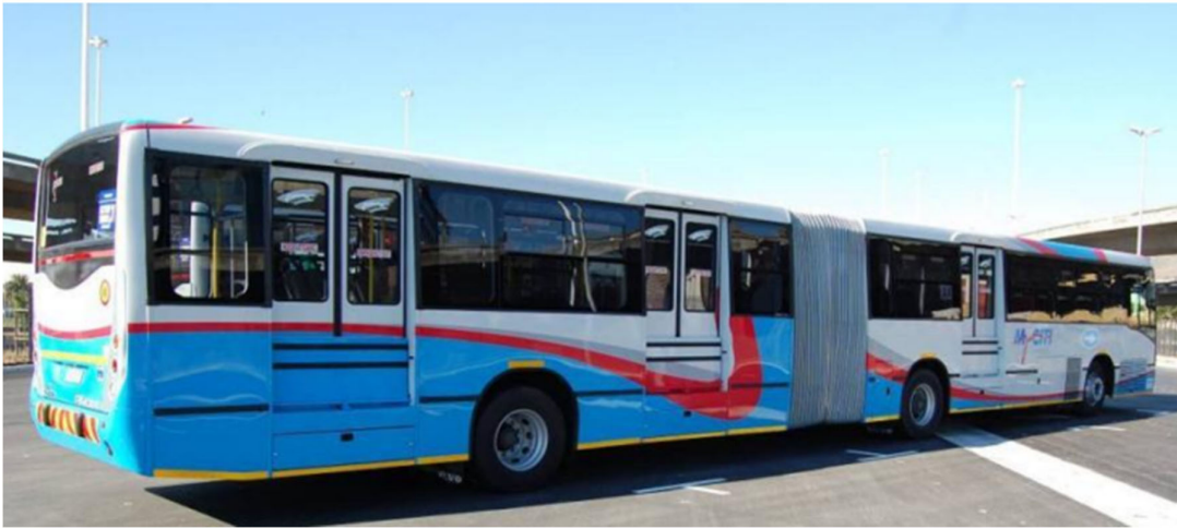
Figure 2-1: Example of a high floor 18m bus
